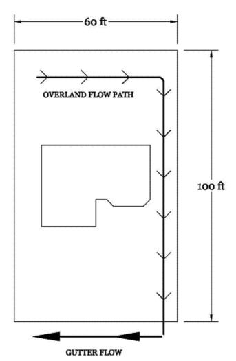
OVERLAND FLOW LENGTH = 160ft TO GUTTER GUTTER FLOW LENGTH = 420ft TO INLET SHED AREA TO INLET = 1.4 ACRES 35% OF SHED AREA PERVIOUS
